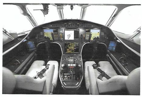
The next enhancement to the FalconEye option will be the addition of a dual head-up display configuration that will support an EFVS-to-land capability, allowing pilots to fly a full approach and land without requiring natural vision to see the runway. The full approval of this capability is anticipated next year.
