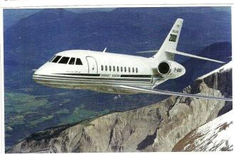
The original Falcon 2000 was the first business jet in the world to be designed using a fully digital mockup, with the Dassault design team responding to Falcon operator requirements in those days, which helped define the aircraft's initial performance, the ideal range (which was a perfect fit for the US 'coast-to-coast' market) and operating costs. Since the original design, there have been six versions of the Falcon 2000, including the 2000LXS introduced in October 2012.
