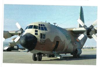
The first improved C-130 ('Karnaf', Hebrew for Rhino) heavy transport aircraft has flown from Nevatim Airbase in southern Israel after a long process in which new and advanced systems were installed on it and its main wing was replaced, as part of an overall renewal project for the C-130 division. It is expected that within a few years, the concerned squadron will only operate the improved C-130s which are to be in service till 2040.
